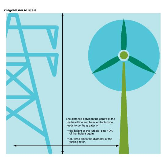
Turbines should be far enough away to avoid the possibility of toppling onto the overhead line
